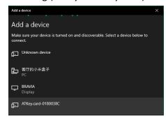
Click target ATKey.card, click "Connect" from UI and touch fingerprint sensor (LED#2 is white flashing) to confirm the pairing
