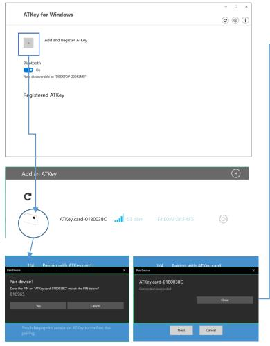
LED#2 is WHITE flashing, touch fingerprint to confirm the pairing, and also click "Yes" from UI.
