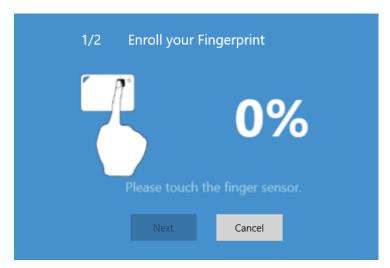
Enroll new fingerprint in by ~12 times touch, following UI message; up to 10x fingerprints
