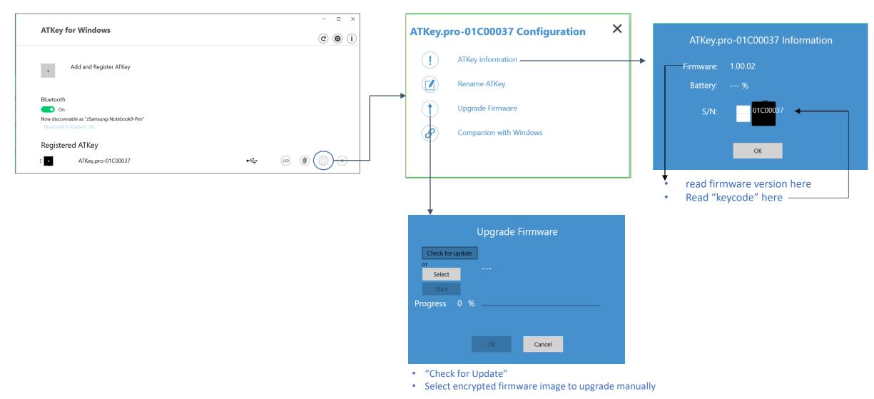
• Please wait till 100% done, then plug ATKey.Pro off USB port; re-insert to USB port, waiting ~15 sec to boot to new firmware (LED from White to Blue ON).
