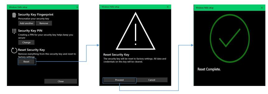
Following UI message, remove and re-insert USB port, all actions need to be done within 10 seconds.
