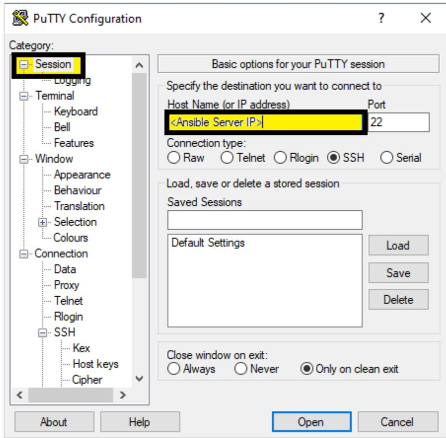
Figure 3: Configure the public IP address and Port
