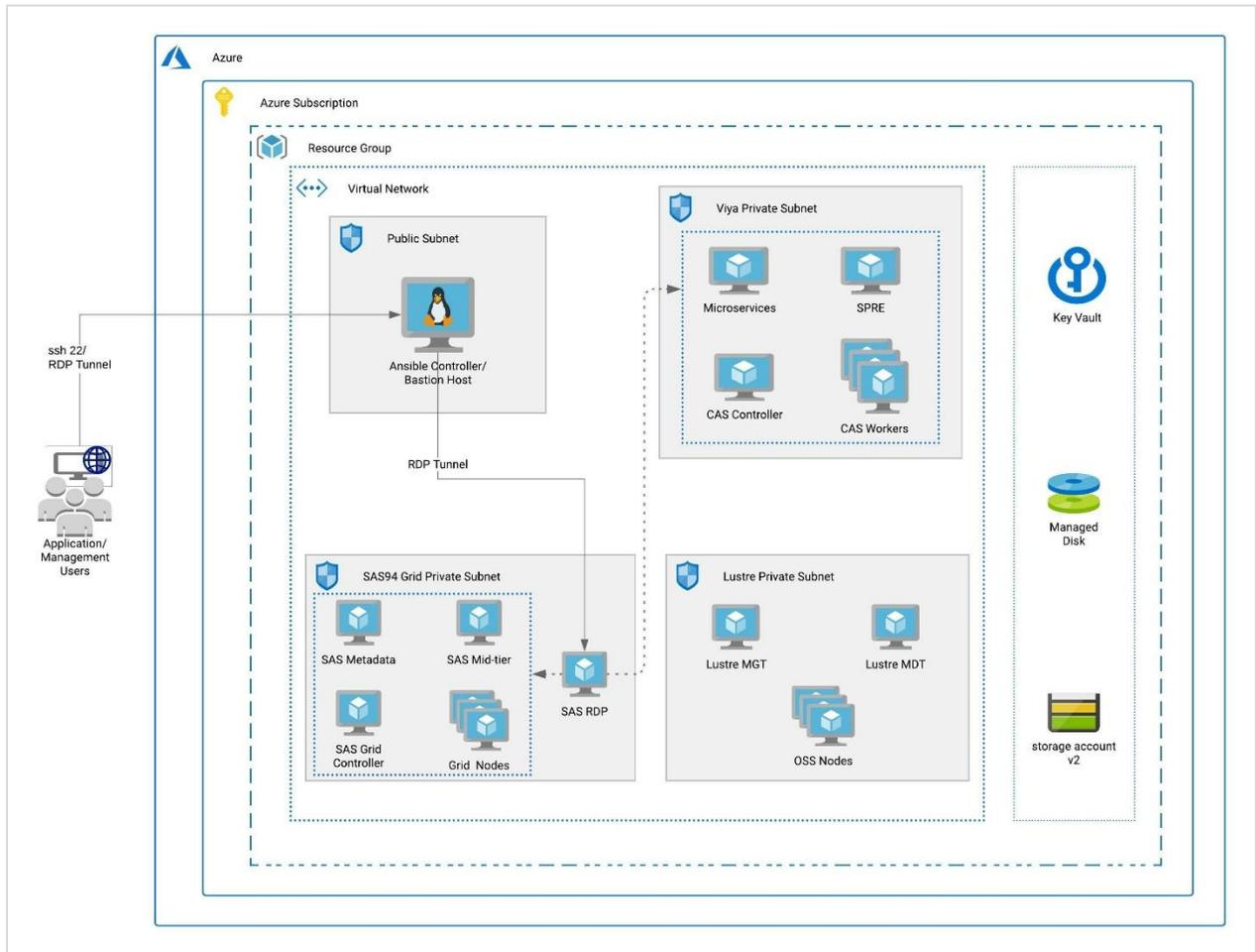
Figure 2: SAS Grid and SAS Viya Architecture Diagram
