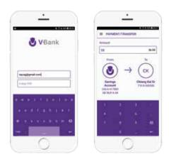
V-Key implements secure keyboards against keylogging in order to provide defense-in-depth against this common attack on mobile applications. For additional threat protection and intelligence, the solution also scans for keylogging techniques using a combination of heuristic checks and signatures.
