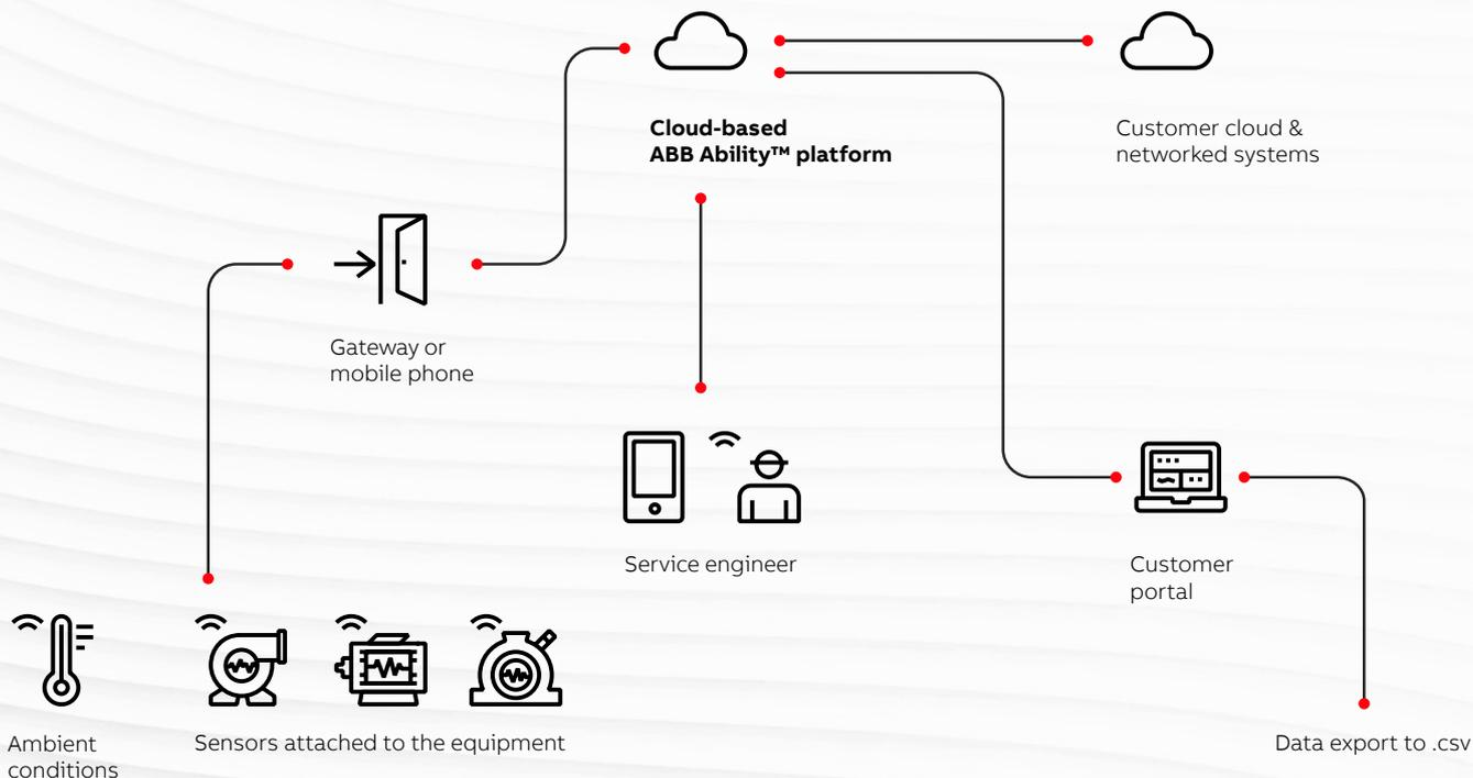
— 01 ABB's condition monitoring solution for LV motors: The ABB Ability™ Smart Sensor transmits data via a smartphone or gateway to a secure cloud service. Algorithms analyze the data and convert it into meaningful information, which is sent to the user's smartphone and customer portal.
