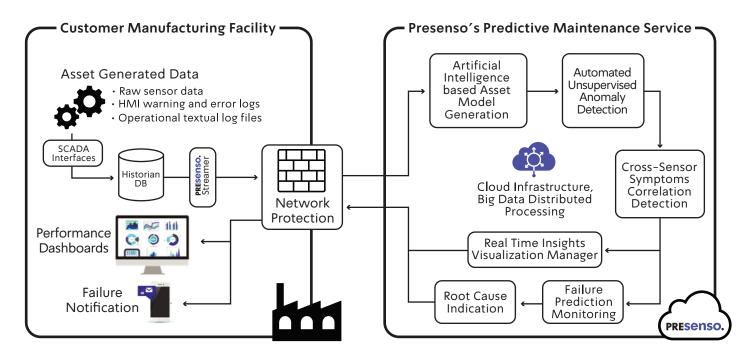
The Presenso Cloud continuously acquires the Big Data generated by multiple sensors that are already installed in industrial manufacturing lines and machines. The real-time streamed-in data is run through an ensemble of unique "Machine Learning" and "Deep Learning" algorithms designed to predict and alert on any upcoming failure.
