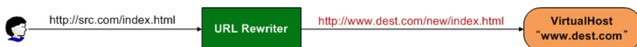
Fig. 5.1: The request can only reach the virtual host by passing through the URL Rewriter.
