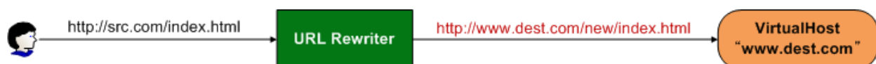
Fig. 3.8: The request can only reach the virtual host by passing through the URL Rewriter.
