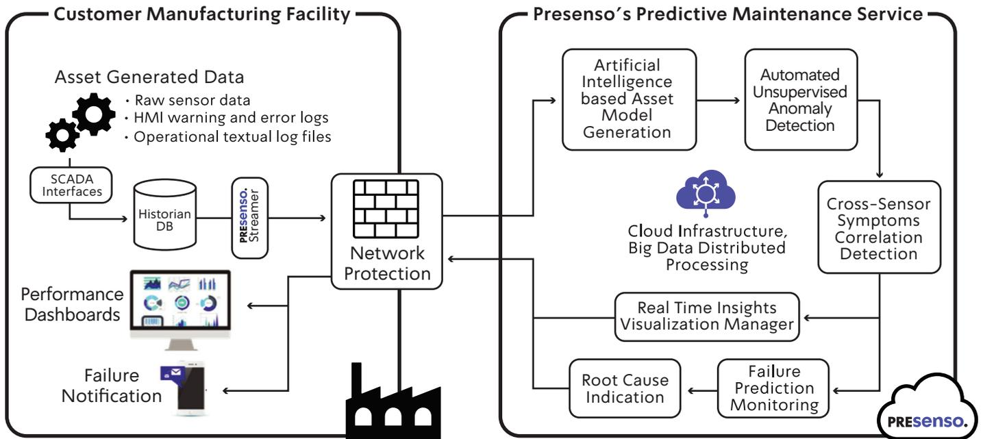
The Presenso Cloud continuously acquires the Big Data generated by multiple sensors that are already installed in industrial manufacturing lines and machines. The real-time streamed-in data is run through an ensemble of unique "Machine Learning" and "Deep Learning" algorithms designed to predict and alert on any upcoming failure.
