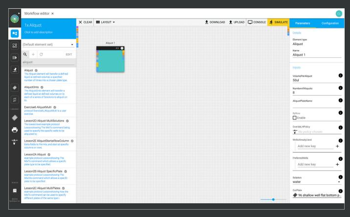
Workflow Editor Workflows are composed of individual 'elements'. Each element contains a specific instruction – in this example, to aliquot. The various parameters of the aliquot can be defined in the right-hand panel.
