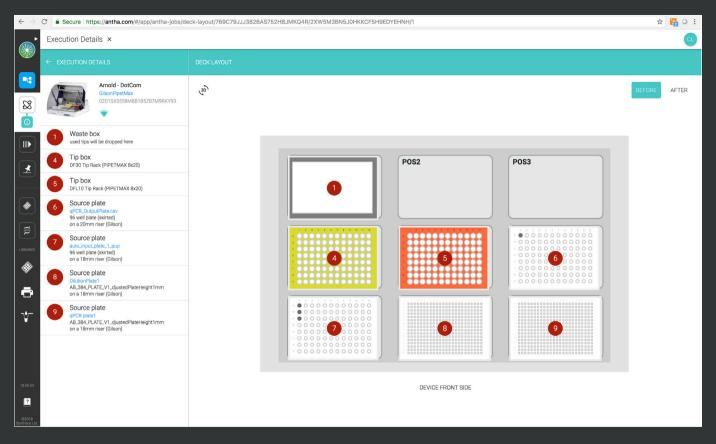
**Deck Layout** Antha tells you where to put your plates, tip box, and waste box on the instrument's deck.
