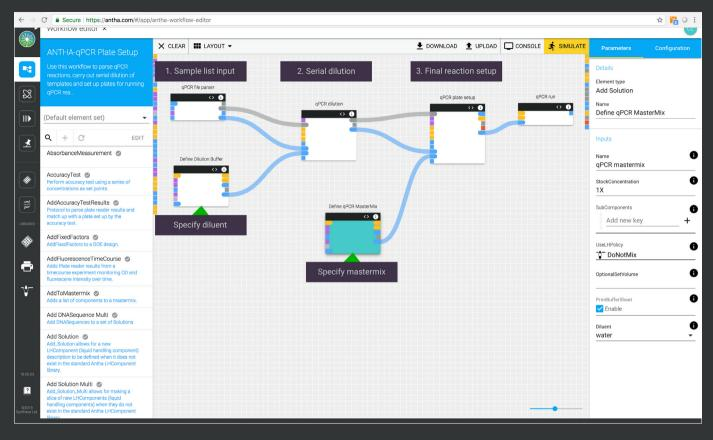
**Workflow Editor** Link the elements together to create your entire workflow. In this example, a qPCR assay set-up.
