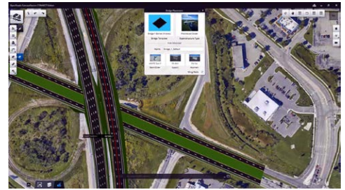
Road design leveraging a reality mesh in Bentley's OpenRoads ConceptStation.
