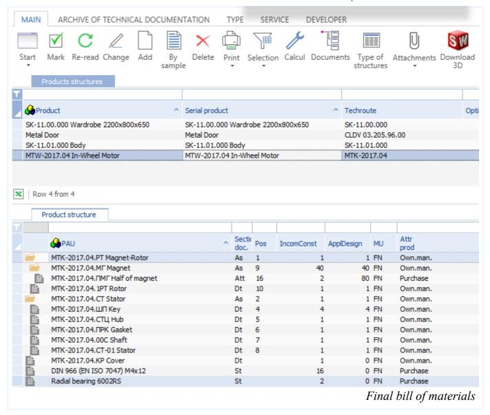
The system functions include setting a method for automatic code generation based on design designation for all items of the bill of materials.
