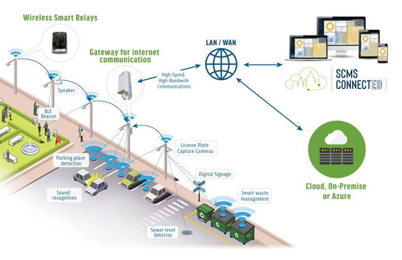
As an example, in smart city projects, radio modules, also called "nodes" are connected to every street light. This creates a powerful and cost-effective wireless mesh network that covers an entire area and that allows to manage every type of IoT device installed over time.
