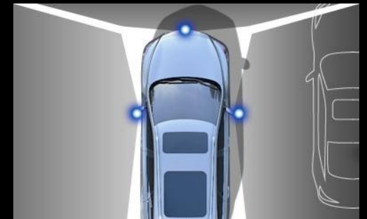
Remote Camera View of Car Environment e.g. Infiniti Around View Monitor
