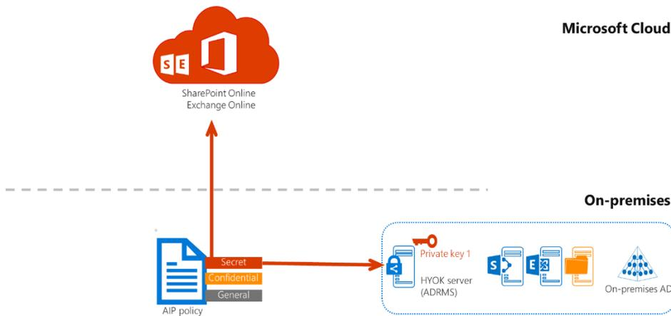
*DIAGRAM - Here is an example of an HYOK topology. Customer has on-premises AD, AD RMS server and HSM. Customer's private keys are managed in the on-premises HSM, and used by the on-premises AD RMS server. The customer physically possesses their private keys and does not share these keys with the Microsoft cloud. The AIP classification labels are bound to the Azure RMS server – so when an end user applies the specific label, which in this example is 'Secret' it will be protected with HYOK.*
