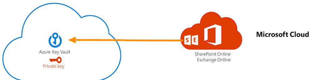
*DIAGRAM - Here is a simplified view of customer managed keys managed in Azure Key Vault. The customer provides and manages their asymmetric private keys in Azure Key Vault. The customers' private keys do not leave Azure Key Vault's HSM boundary and customers have the control to revoke their private keys to make the data inaccessible to the service, and initiate the path towards data deletion.*
